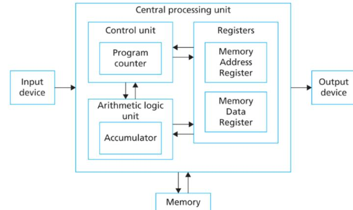
**Control Unit (CU):** executes instructions and controls the flow of data in the CPU.
