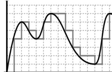
The analogue wave is smoother and shows continuous data. The digital sampling shows the amplitude of the wave at different points.
